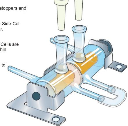
We have chosen to illustrate the flow moving through the cell in one direction, but either direction is acceptable.
