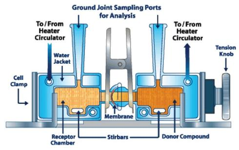
You can choose from one of the joint 3 O ring, ground plane, the plane flange in addition to fit. Ground plane is used most commonly, as a Dialysis membrane if it be a film of the plane It does not leak when many also occur in a very thin film.
